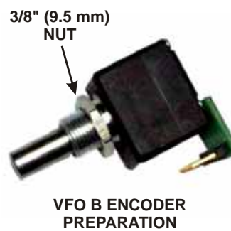
Figure 38. Preparing VFO Encoders for Mounting.
