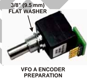
Figure 38. Preparing VFO Encoders for Mounting.
