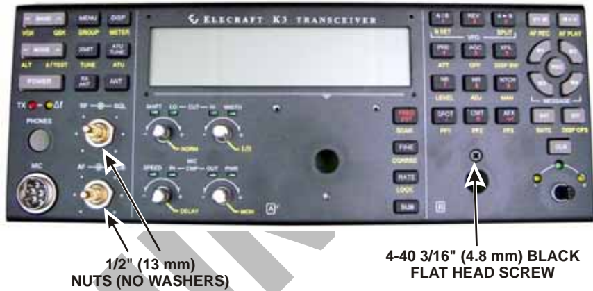
Figure 37. Mounting the Front Panel on the Front Panel Board.
