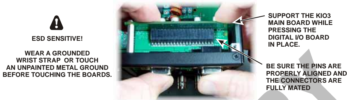
Figure 33. Installing the KIO3 Digital I/O Board.
